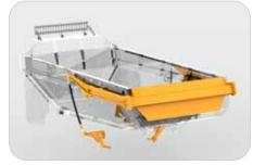
A tailgate is available as an option for better material retention. The tailgate opens as the bin is raised for dumping. Unlike chains, the spring steel straps in a Bell ADT bin maintain a positive seal throughout the haul ensuring minimal material is lost.
