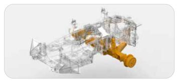
For comfortable productivity, the A-frame suspension system coupled with hydropneumatic suspension struts reduce the discomfort of lateral vibration often experienced with off-road conditions. A superior suspension seat provides additional isolation for the operator.
