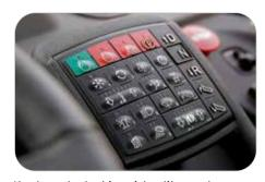
Keyless start, driver identity and access codes ensure no unauthorised operation of your equipment.
