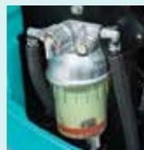
Pre fuel filter with built-in water separator
