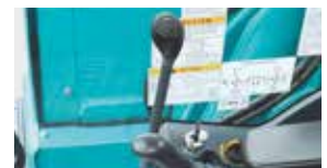
• Travel speed select switch The switch is equipped with the dozer lever.
