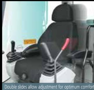
Double slides allow adjustment for optimum comfort
