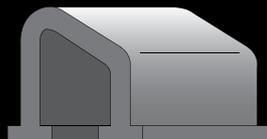
Special crawler frame design for easy mud removal cleaning.
