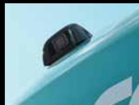
A rear view camera is installed as option to simplify checking for safety behind the machine. The picture appears on the monitor.
