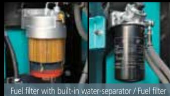
Fuel filter with built-in water-separator / Fuel filter
