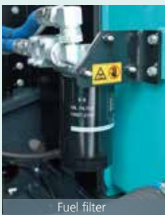
Fuel filter with built-in water-separator
