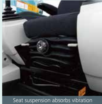
Seat suspension absorbs vibration
