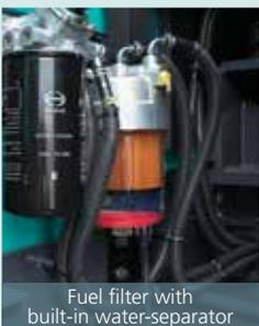
Fuel filter with built-in water-separator
