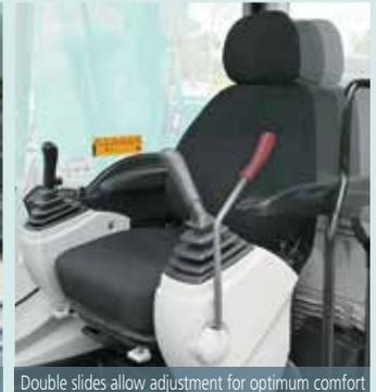
Double slides allow adjustment for optimum comfort
