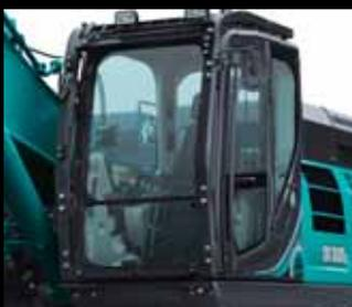
ROPS (Roll-Over-Protective Structure)-compliant cab clears ISO standards (ISO-12117-2: 2008) and ensures greater safety for the operator should the machine tip over.
