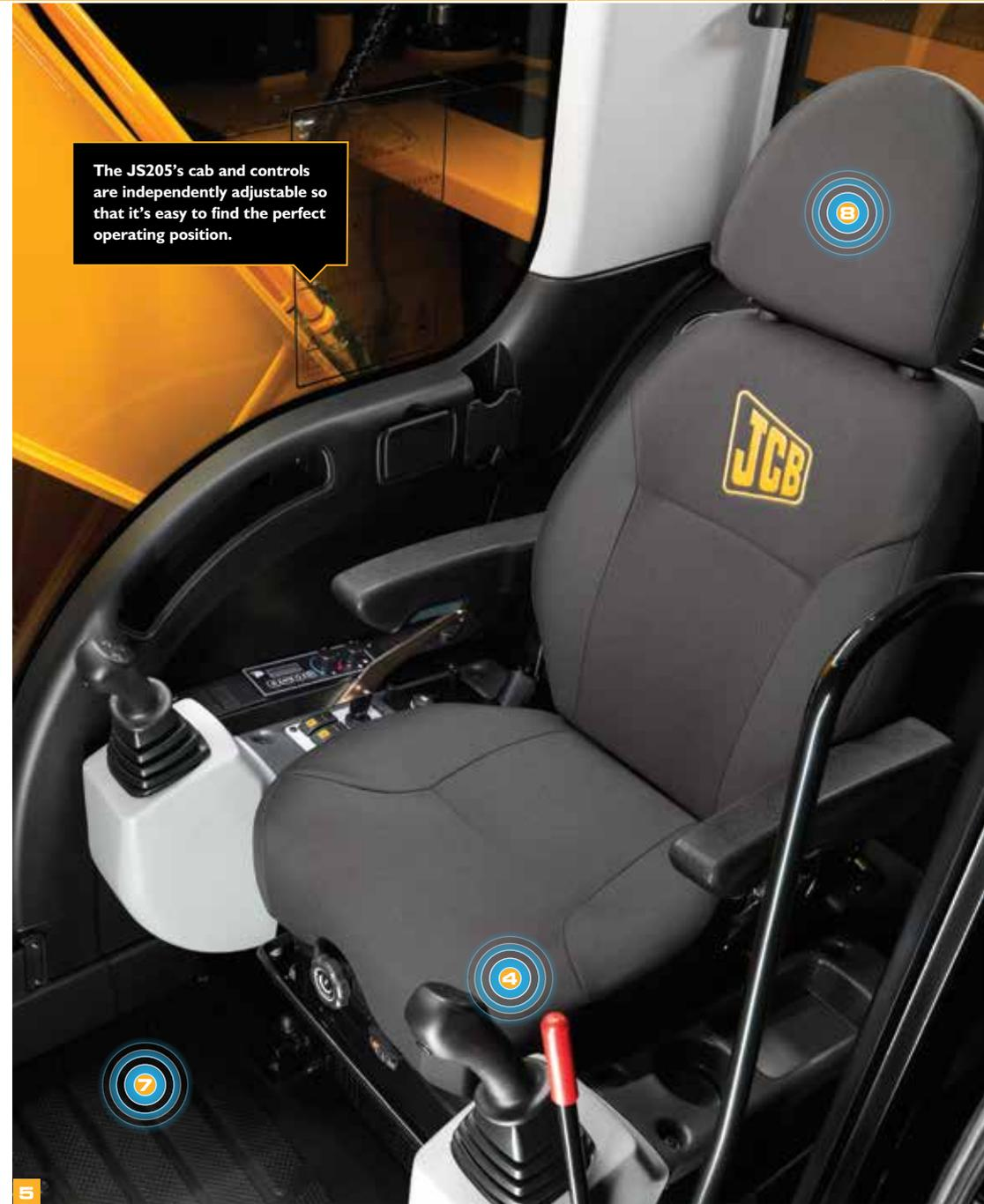
The JS205's cab and controls are independently adjustable so that it's easy to find the perfect operating position.
