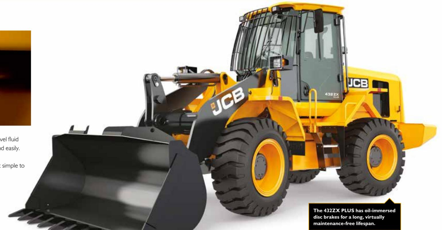
The 432ZX PLUS has oil-immersed disc brakes for a long, virtually maintenance-free lifespan.
