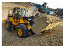
Class-leading climbing and stockpiling capability with high power-to-weight ratio and 27° departure angle. Z-Bar loader design delivers 188kN of breakout force.
