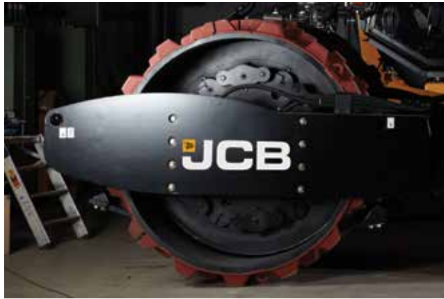
Quick and easy fitting of padfoot shell segments (3 segments). Kit comes with scrapers.
